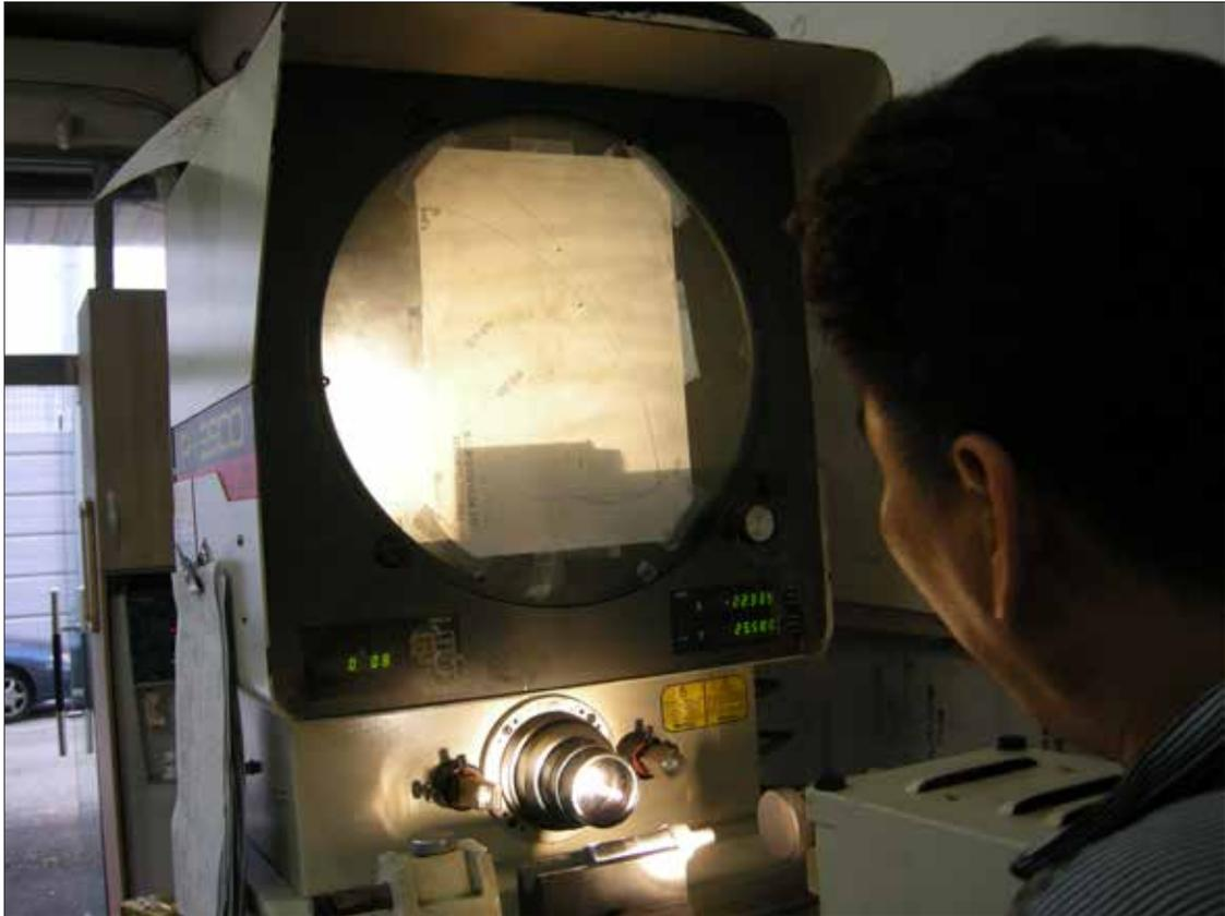
The photos above and below left show an optical comparator in use to assure that our parts match our new specification tolerances which must be held closer than ever before.
